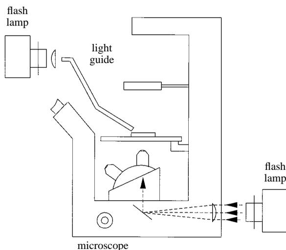
Fig. 4. Light can be focused directly onto a preparation, or directed through a liquid light guide or the optical path of a microscope. From Gurney (1993).
