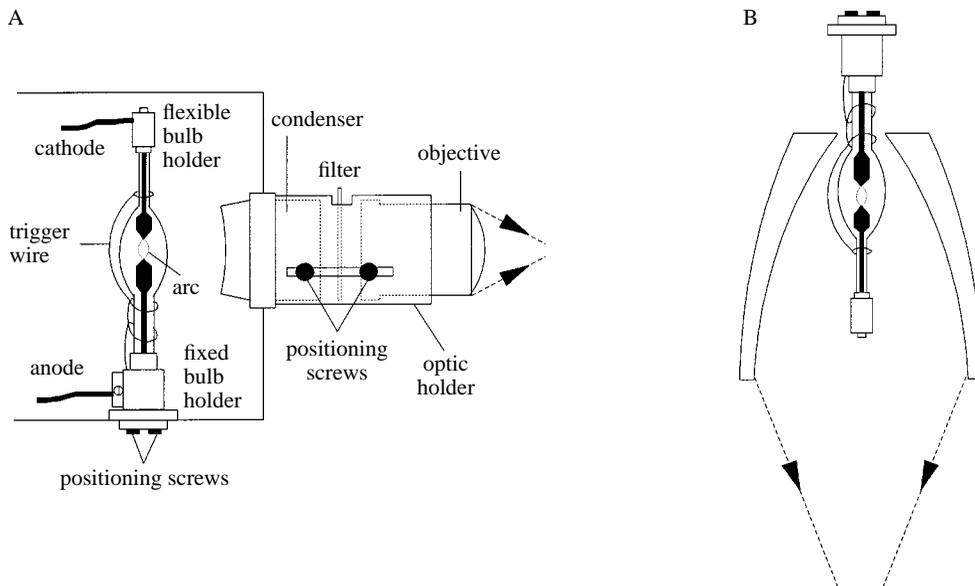
Fig. 3. (A) Diagram of the optical arrangement inside the lamp housing of a standard Rapp flashlamp, illustrating the use of a quartz condenser and objective to focus the light spot. From Gurney (1991). (B) An ellipsoid mirror arrangement to focus the light.
