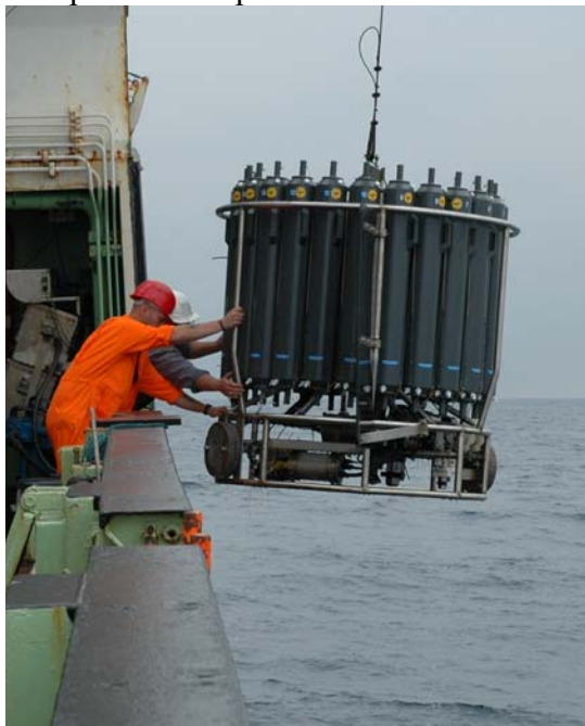
FIGURE Lowering a CTD from the side of a ship.
