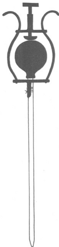
Fig. 11. Simple automatic pipette used for adding reagent while shaking contents of flask, showing rubber ball on glass pipette and plunger with limited travel adjusted to suck in and deliver the required quantity.
