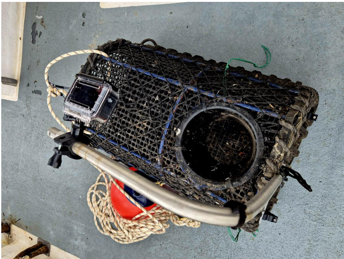
Figure 5.1. The setup used to film species interactions with a shellfish parlour pot. The camera is a DJI Osmo Action 4 which was normally set to time lapse with an image taken every 15 seconds.
