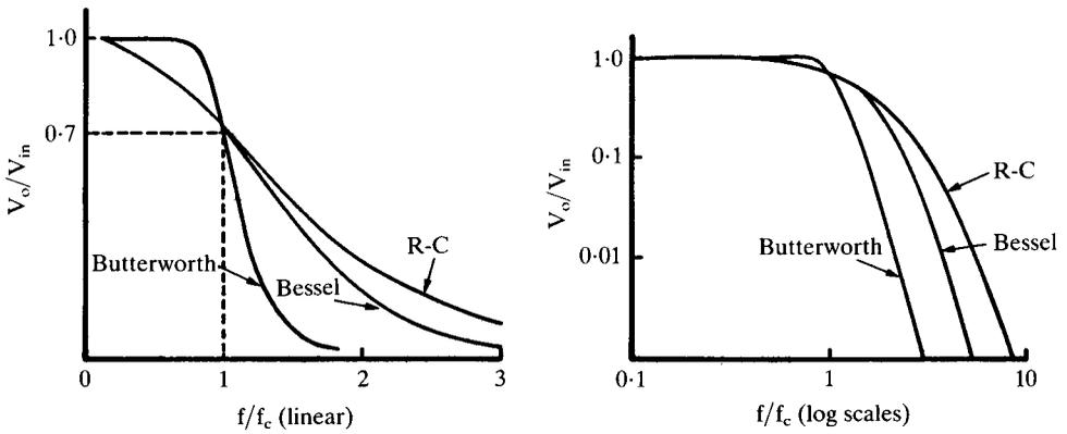
Fig. 4. Comparison of filter characteristics for  $n=6$ .
