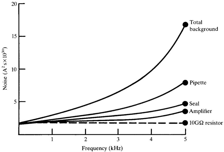
Fig. 9. Contribution of noise from different sources. From Sigworth (1983) with permission.
