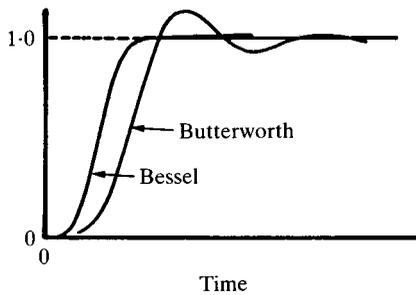
Fig. 5. Response of Butterworth and Bessel low pass filters ( $n=6$ ) to a step input at  $t=0$ .
