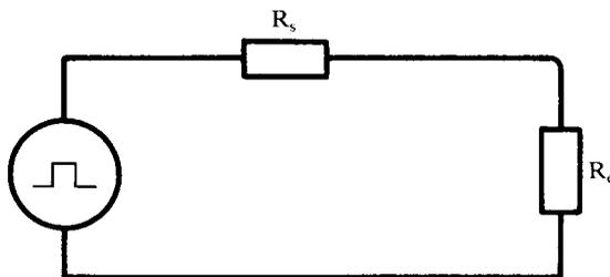
This arrangement works for small currents. With large currents, a capacitive transient may occur due to conduction of the rapidly rising edges of a rectangular pulse over the parallel capacitance of the large value series resistor.
