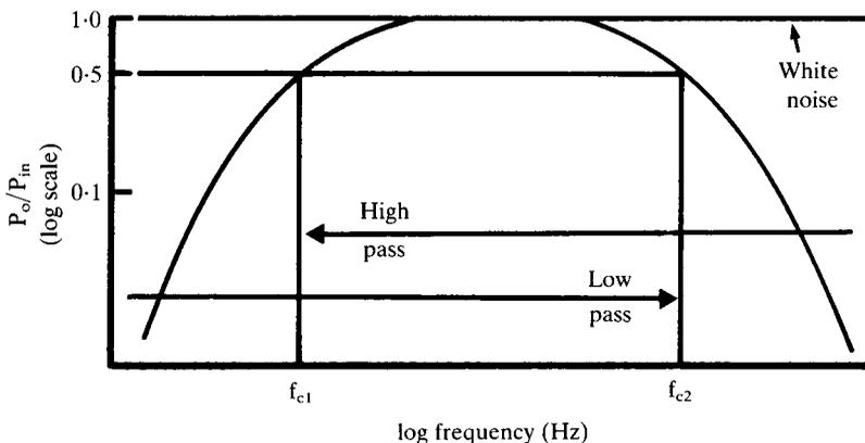
Fig. 1. Power spectrum to show high ( $f_{c1}$ ) and low ( $f_{c2}$ ) pass filtering of white noise input.
