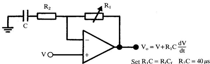
This operates as a voltage follower at low frequencies but increases in gain at high frequencies. Time constant  $R_1C$  is adjusted to the same value as that produced by stray feedback capacitance in the I/V amplifier;  $R_2$  provides damping to prevent oscillation. If the patch clamp input stage amplifier has a more complicated response, as is the case with commercial switchable resistor designs, then additional waveform shaping circuits are used to compensate the response.
