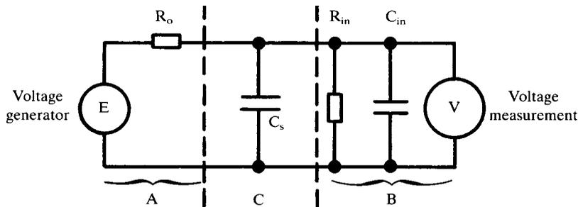
A. *Source of voltage.* The potential  $V$  is developed across the output of a voltage generator represented by an ideal voltage source  $E$  in series with a small output
