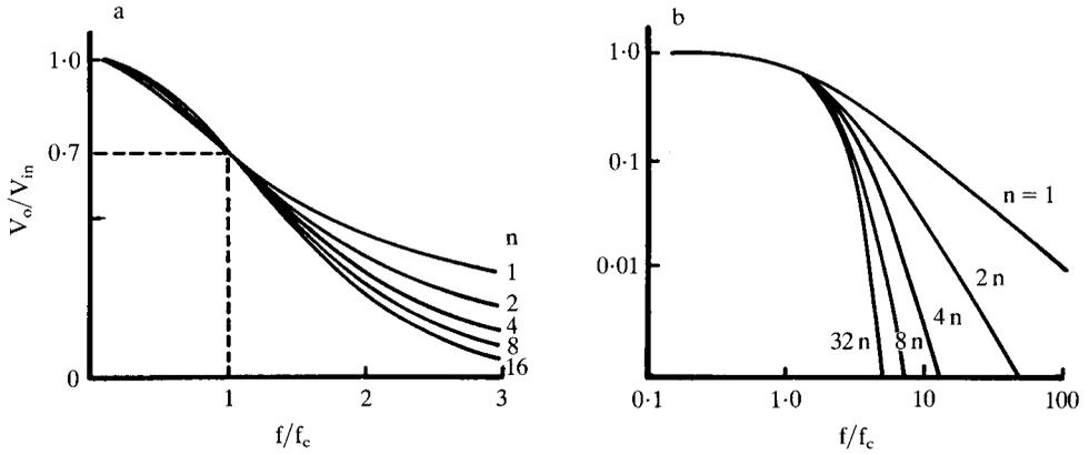
Fig. 3. Cascade R-C filter sections. (a) In the region near  $f_c$  on a linear scale. (b) On log coordinates.  $n$  is the number of cascaded sections (poles).
