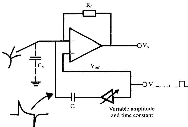
$C_p$ =stray pipette capacity,  $C_i$  is the capacitor for injection of compensation current.
