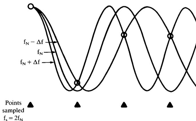
Fig. 6. Aliasing of  $(f_N + \Delta f)$  with  $f_N - \Delta f$ .
