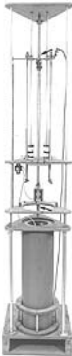
Left: Fig. 18. Deep plunge-freezer, overall height 2.25 m.
