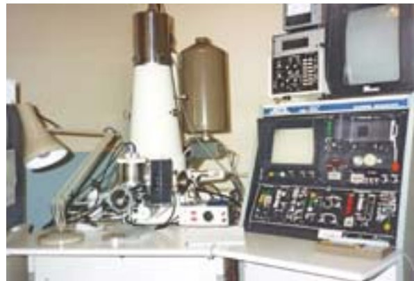
Above: Fig. 12. JEOL 35C SEM in its original location in the basement, with the cryo-stage attached to the airlock and the brown dewar of the x-ray detector at the rear of the column. The x-ray system was controlled very easily by the small keypad at the right side of the microscope console. The microscope was moved upstairs to Room 57 in 1988.
