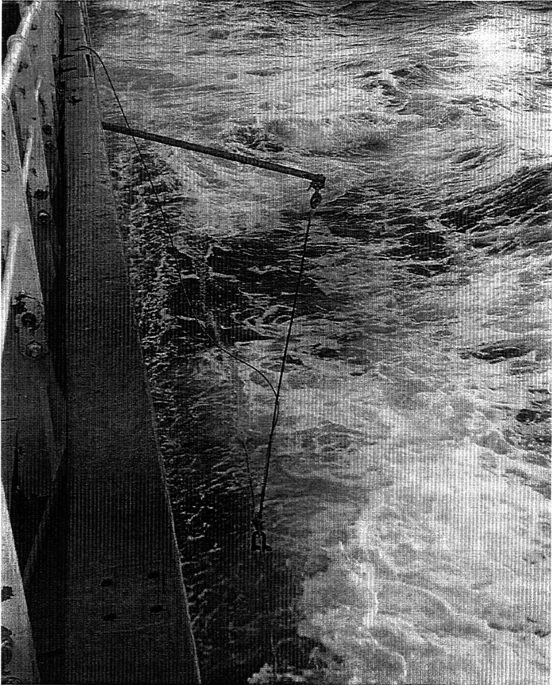
Figure 2. IOS SOAP sensor as deployed on the James Clark Ross during AMT-7/ROSSA 1998.
