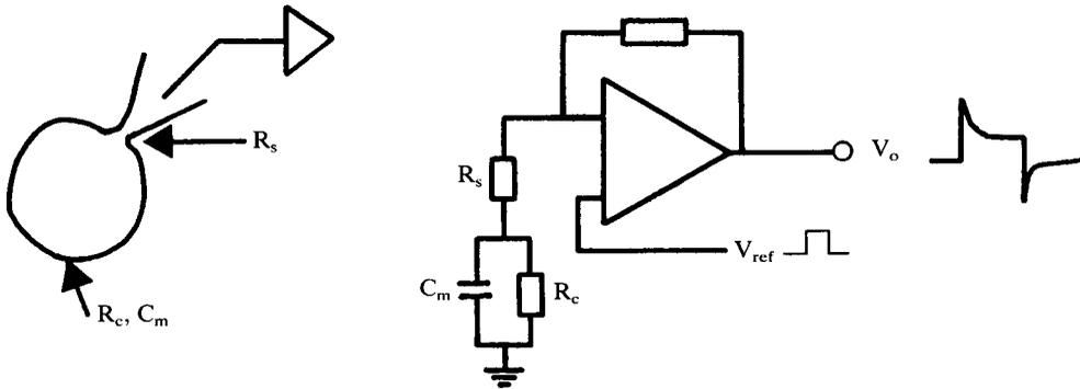
Voltage pulses to  $V_{ref}$  (and hence the pipette) cause current to flow into the cell through  $R_s$  to charge the cell capacitance,  $C_m$ . This gives rise to a current output with initial transients of time constant
