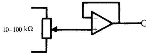
but gains of 10 or more may be used as described above. If good quality operational amplifiers are used, the voltage follower configuration may be used in microelectrode amplifiers.
