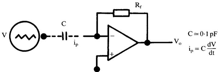
*Setting the gain:* this is done by connecting a precisely know resistance (about 100 MΩ) between input and ground, applying a voltage step V to the non-inverting ( $V_{ref}$ ) or command input to give  $i_p = V/R$  and looking at the output deflection  $V_o$ :
