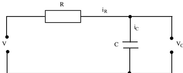
Current flowing into the capacitor is supplied via the resistor, so currents flowing *into* the junction (defined positive) of  $R$  and  $C$ , where the voltage across the capacitor is measured, are
