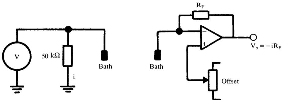
A better arrangement is the virtual earth circuit discussed above, which has the advantage that the bath potential is clamped at a constant level (set by the offset circuit), provided currents are not so large that polarization of the bath electrode occurs. The sensitivity is now set by the value of  $R_F$ ,  $V_O = -iR_F$ , without affecting the bath potential, and practically may be 1 or 10 mV/nA ( $R_F = 1 \text{ M}\Omega$  or  $10 \text{ M}\Omega$ ).
