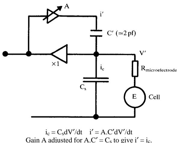
Fig. 8. Capacity compensation.
