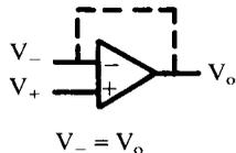
If the open loop gain is  $A$ , then  $V_o=A(V_+-V_-)$  and, since  $V_-=V_o$ ,  $V_o=V_+A/(1+A)$ . Therefore, if  $A$  is large,  $V_o\approx V_+$  and  $V_-\approx V_+$ , i.e. to a good approximation the output follows the input,  $V_+$ , and voltages on (+) and (-) are equal. By applying only a proportion, say  $1/x$ , of  $V_o$  to  $V_-$ , a circuit with gain= $x$  is produced. In this case  $V_o=A(V_+-V_o/x)$  which can be rearranged to give
