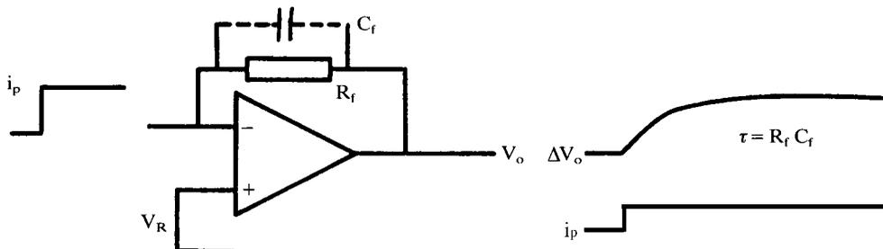
Provided parallel capacity is uniformly distributed over the resistor the response is approximately a single exponential. The output voltage for a step input of current  $i_p$  is
