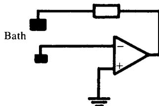
Current measurement within a circuit is also achieved with an inverting amplifier.
