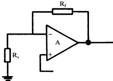
(1) The (-) input is connected to ground via  $R_s$  (seal and bath) and  $R_f$  (amplifier output). The source (seal) resistance  $R_s$  and feedback  $R_f$  give rise to voltage noise of approximately
