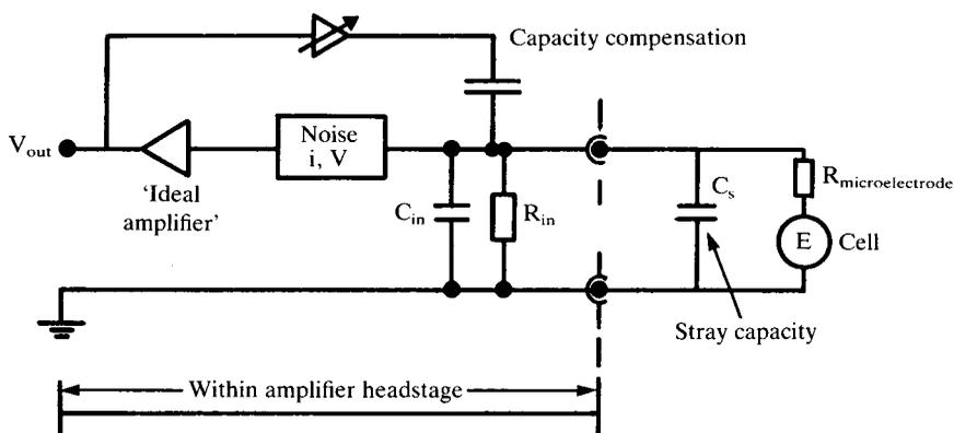
Fig. 7. Schematic diagram of microelectrode amplifier headstage and microelectrode.
