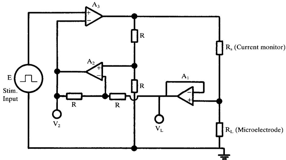
$$V_2 = IR_s \quad V_L = IR_L$$
