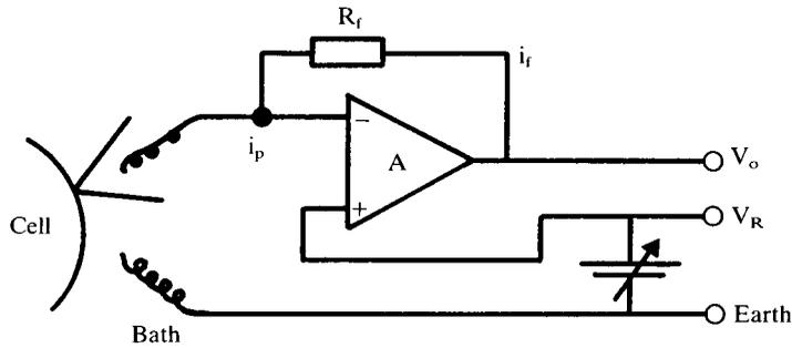
where the amplifier A maintains the (-) input at the same potential as (+) i.e.  $V_R$ , by negative feedback through resistor  $R_f$ . Thus, if the current flowing into (-) is neglected,  $i_p + i_f = 0$  and  $(V_O - V_R) = i_f R_f = -i_p R_f$ .
