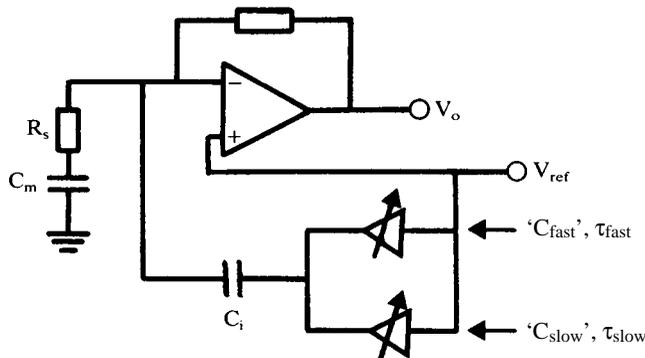
Unlike a microelectrode amplifier, the use of slow capacitance compensation does not improve the speed of clamping the cell membrane potential (unless the amplifiers have reached saturation) but simply removes the capacitative transient from the
