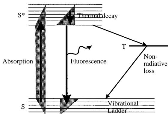
Fig. 1. An energy level diagram for fluorescence excitation. Note the presence of multiple vibrational levels around the principal energy levels S and S\*.
