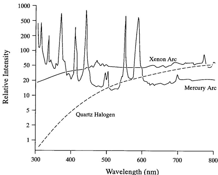
Fig. 6. Comparison of typical spectra of xenon, mercury and quartz halogen light sources. Note that the halogen source is the most uniform but the output drops quite rapidly in the violet and is not useful for UV illumination. The xenon arc source has a smoother spectrum than the mercury arc, but the sharp peaks of the mercury spectrum can be useful if they occur at desired wavelengths.
