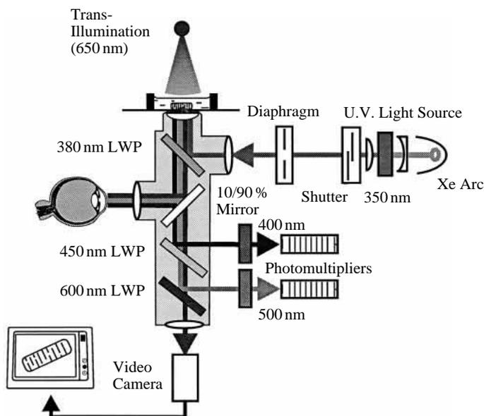
Fig. 3. A schematic diagram of an inverted epifluorescence microscope system for indo-1 fluorescence detection. For fura-2 this system would have to be modified to include some method for changing excitation wavelength. The LWP (long wave pass) mirrors are dichroic mirrors that split the light at the wavelengths indicated. Note that red light (650 nm) is used to give continuous illumination of the preparation, so that it can be observed by eye or via a camera.
