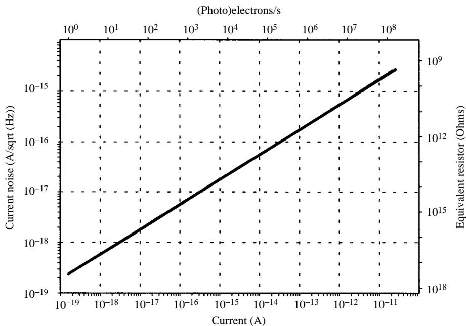
Fig 5. The relationship between current flow and shot noise at 25°C. The top of the graph shows the electron flow rate and the value of the resistor that gives the same noise level is shown at the right axis. Note the large resistor values that would be required to reproduce shot noise.
