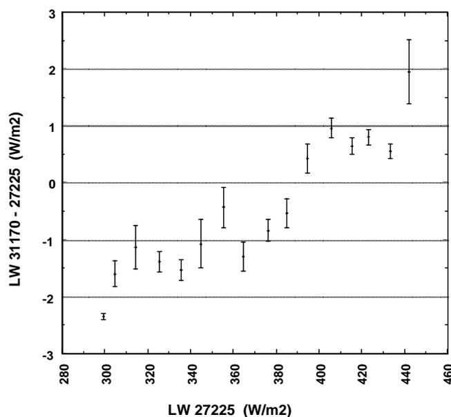
**Figure 8.** The difference in longwave radiation from the two pyrgeometers. The error bars indicate the standard deviation of the mean.
