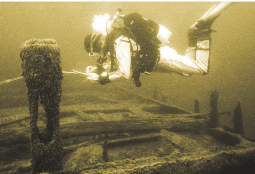
FIGURE 4a-b Photo of the bilge pump of the Björns wreck from 2003. The picture taken in 2008 shows its subsequent collapse, probably due to divers or anchoring. Photo: Mirja Arnshaw and Patrik Höglund, SMM
