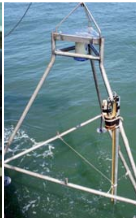
FIGURE 3 LEFT: LAB TESTING OF THE 'SEAGRASS' INSTRUMENT IN SEDIMENT FLUMES (FLANDERS HYDRAULICS RESEARCH). RIGHT: THE PLACING OF A MEASURING ROD OFF-SHORE © RCMG
