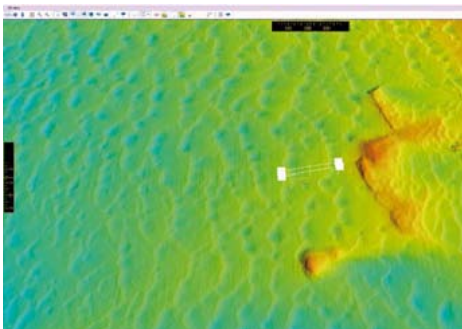
FIGURE 3 A multibeam image of the site showing clear man-made structures. Source: RWS
