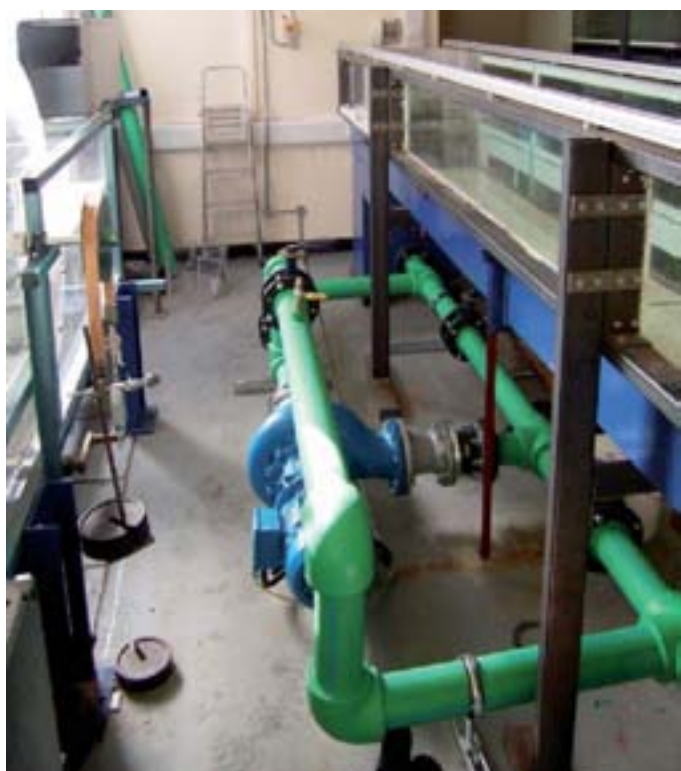
FIGURE 1a-b Bi-directional pump system and the placement of the model vessel on the mobile bed. The coins and blocks represent reference points to enable stitching of laser scans so larger surface areas can be recorded.
